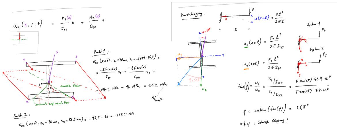
Figure 1: Part of notes showing an exercise of superposed stresses in a cantilever beam (unsymmetrical) bending.
