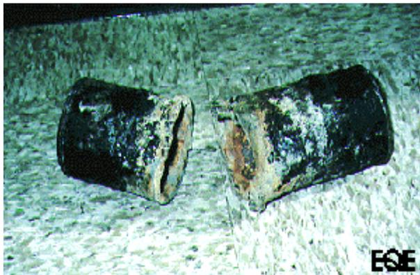
**Failure along the welding seam of an 8 cm diameter gas pipeline**
