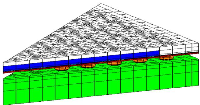
**Examples of CAD-use in microelectronics modeling: FE-meshes for a CSP**
