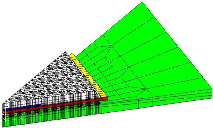
**Examples of CAD-use in microelectronics modeling: FE-meshes for a BGA**
