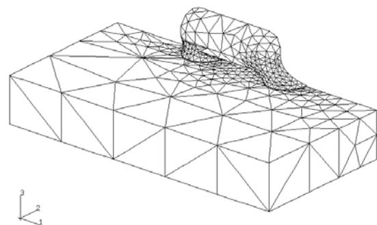
**Examples of CAD-use in microelectronics modeling: FE-meshes for a MiniMELF**
