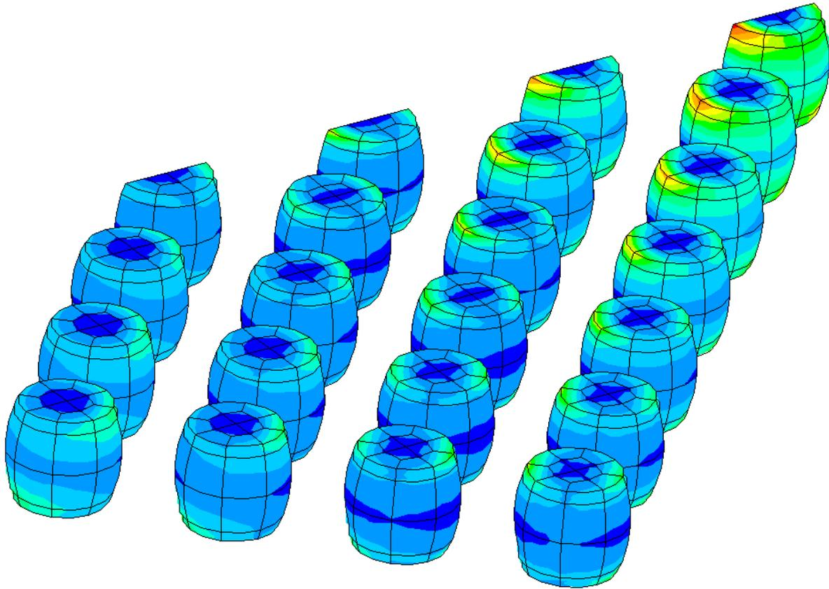
**Accumulation of creep strain in the solder bumps of a CSP as a consequence of thermal cycling.**
